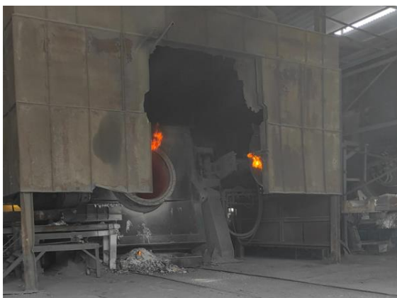
Figure 27. Left, furnace for primary melting; right, furnace for secondary melting and alloying
