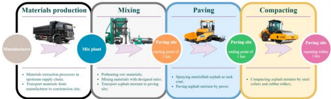
Figure 6: Asphalt production, transport and application.
