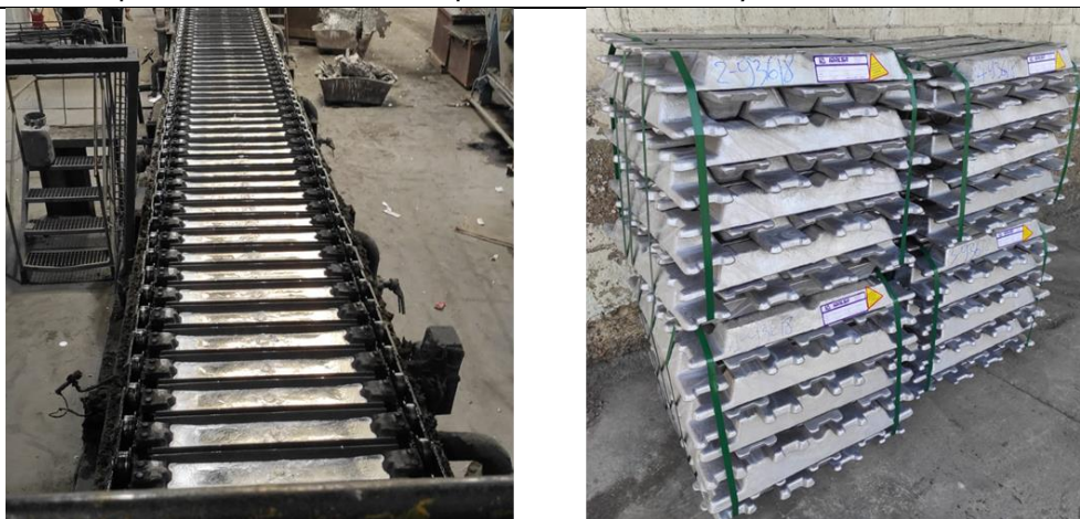
Figure 28. Left, aluminium moulds; right, aluminium billets
